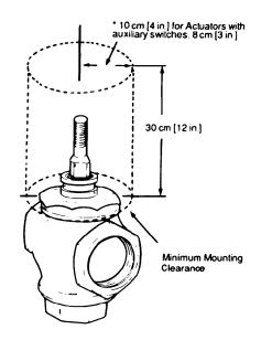
FIG.2 -- MINIMUM MOUNTING CLEARANCE.
